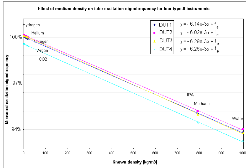
Figure 6.3 Instrument eigenfrequencies with various fluids (media densities)
